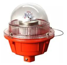
The Low Intensity light is currently available in both single and double configurations operating at a range of 110~240VAC and also in range of 12~48VDC. Both configurations are available as original equipment or as a direct replacement of existing L-810 incandescent lights.
